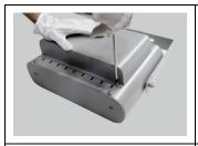
1. Disconnect the luminary from AC power. Unscrew the screws to remove the driver cover.
